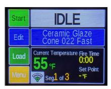
**Control:** Full digital touchscreen Genesis Mini control with easy-to-use interface, WiFi enabled app, and simple programs for firing ceramics or glass.
