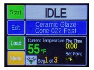
**Control:** Full digital touchscreen Genesis control with easy-to-use interface, WiFi enabled app, and simple programs for firing ceramics or glass.
